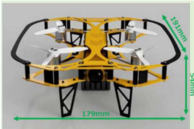
Fig. 9 Investigation equipment for dry area surveillance inside Unit 1 PCV 25
