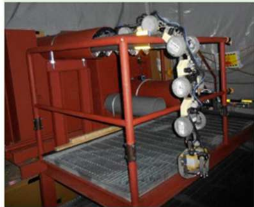
Fig. 9 Investigation equipment for dry area surveillance inside Unit 1 PCV 25
