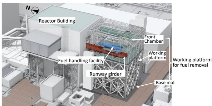
Fig. 10 Fuel removal method in Unit 2 SFP
