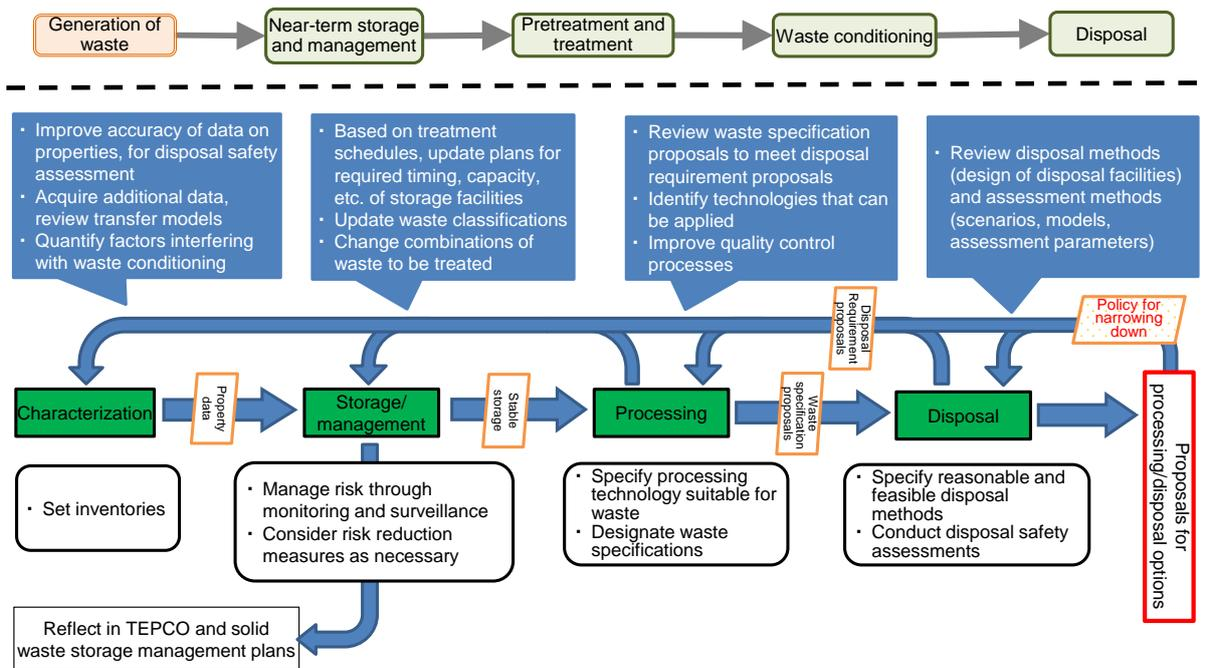
Fig. 7 Procedure to reasonably select safe processing/disposal methods of solid waste
