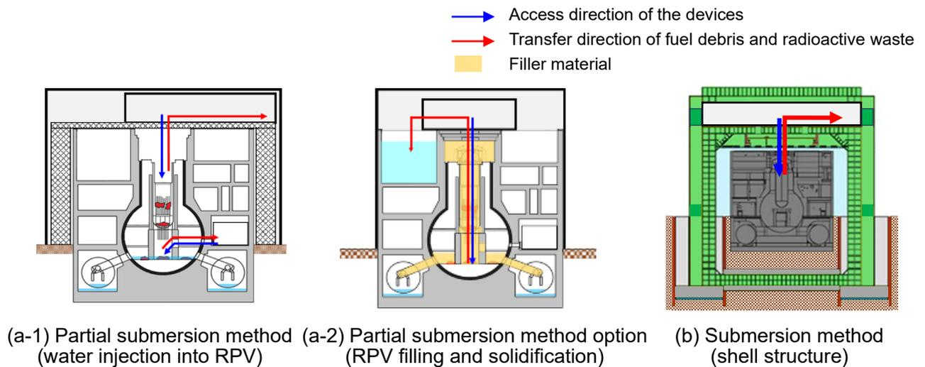
Fig. 6 An example of each retrieval method for further expansion of fuel debris retrieval in scale
