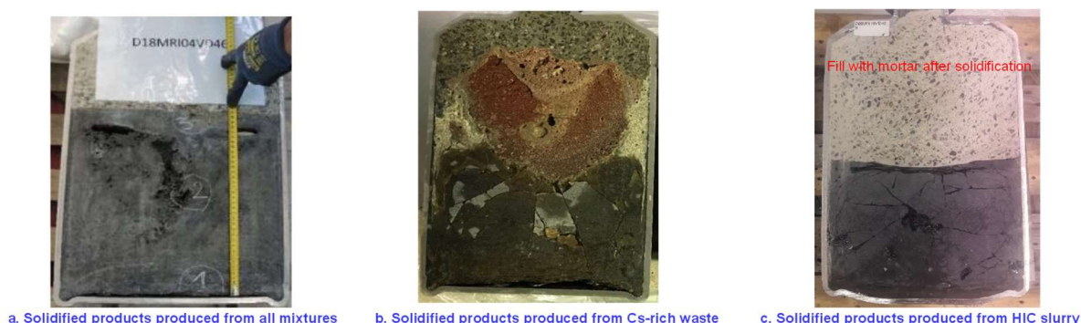
Fig. A11-17 Condition of solidified waste produced by In-Can engineering-scale testing
