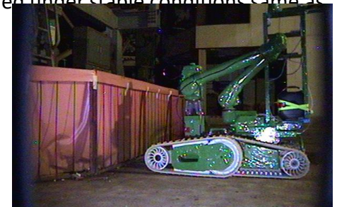
Dose measurement of operation floor of Unit 2 by remote robot (Photo/video library: TEPCO)
